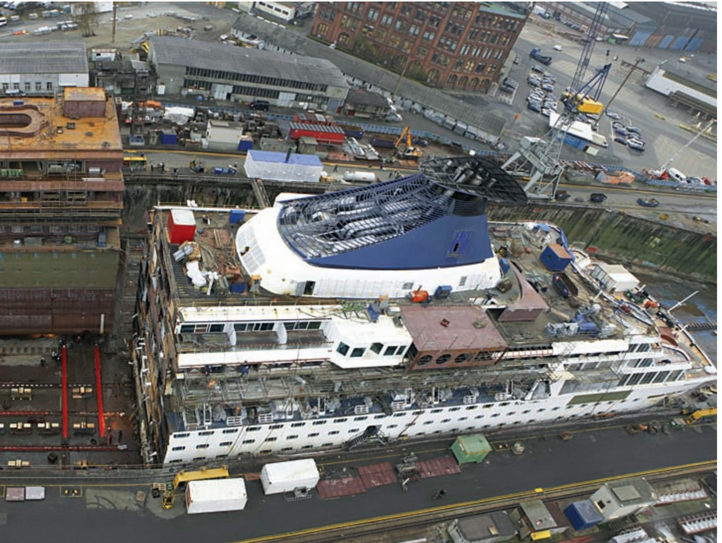
After being cut in half first, the “Norwegian Crown” is lengthened in the “Elbe 17” dry dock by adding a midsection that is 30.20 meters long. The ship will be renamed “Balmoral” once it has been converted and be able to take on 329 additional passengers.
